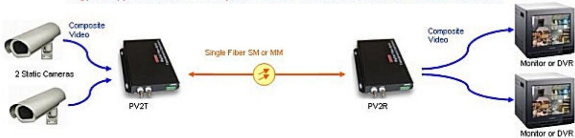
Typical application: 2 channels Upstream Video from 2 static cameras to standalone receiver
